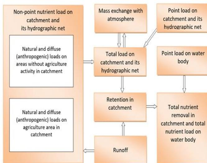
Fig. 7. Schematic picture of the load model ILLM.
